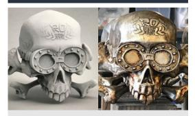
Thingergy's finishing process depends on the desired use. They primarily print in PLA filament, but also use ABS and TPU and occasionally PVA for dissolvable supports. Some prints are coated with Smooth-On's XTC before being body-shopped, primed, and painted. On other projects they body-shop and mold the prints, and then cast in other materials that are sometimes more flexible or durable.
